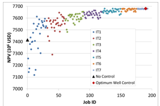
Figure 1: Evolution of the NPV over the simulation jobs for well control optimization in all iterations (IT).
